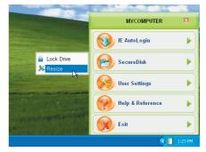
2. You may change the size of the drive by dragging the slider or by typing in an exact size specified in megabytes. The space used by the secure drive is taken from your C: drive and immediately unavailable for other purposes, so pay attention to the available free space on your computer. Click Resize when you are ready to apply the changes.
